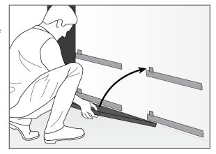
Remove Panel: Lift to remove the panel with the Z-clip now adhered.
