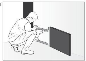
Install Third and Fourth Cleats: Line up your panel again to gauge the placement of the next 2 cleats. These cleats should be placed farther from the screen but at the same heights as the previous ones. (You should be able to secure these next two cleats into studs.)
