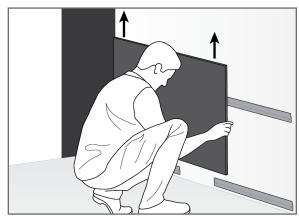
Secure Z-Clips: Secure each Z-clip to the panel using the short screws provided.
