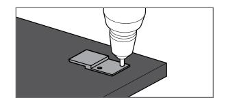
Repeat for All Ceiling Panels: Repeat this process for all ceiling panels, working from the screen and away. Align each panel evenly with adjacent ones and use cleats to attach every panel with four Z-clips in the four corners.
