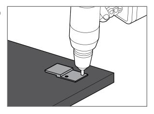
Reinstall Panel: Set the panel back into position onto the cleat.
