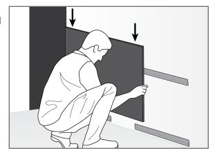
Repeat for All Wall Panels: Repeat this process for all wall panels, working from the bottom to the top, close to the screen, and then outward. Align each panel evenly with adjacent ones and use cleats to attach every panel with four Z-clips in the four corners.
