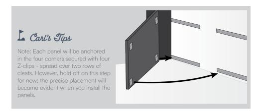
Plan Cleat Placement: Develop a clear plan for positioning your cleats to ensure that each cleat spans the seam of two adjacent panels.
