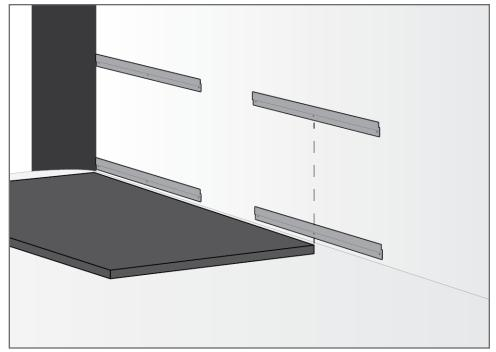
While there's some flexibility in their placement, ensure that the edge closest to the screen sits at least 2" behind the panel, with the remaining part extending beyond the panel to accommodate the installation of the next panel.
