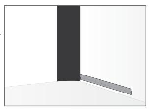
Cleat Orientation: Position the cleat with the grooved edge against the wall, facing downwards, creating space on top for the Z-clips to rest.
