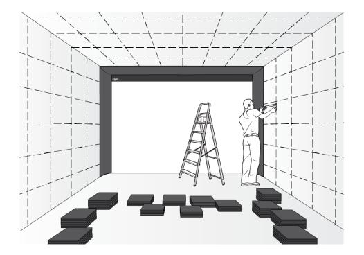
Plan Panel Placement: Line up all your panels on the floor and make sure spacing looks correct prior to installing. This is to help you decide where you want to leave your seam allowance, and where to install the cleats.
