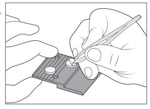
Z-Clip Arrangement: Set a Z-clip into each cleat, four Z-clips in total.
