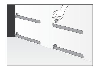
Space the Z-Clips: Measure the Z-clip spacing to align with the panel's width, leaving approximately one inch on each side.
