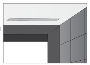
Ceiling Panel Installation: Install ceiling panels in the same manner, starting at the screen and working away from it. Begin by placing the Z-clips with exposed adhesive, then press the panel onto the adhesive.
