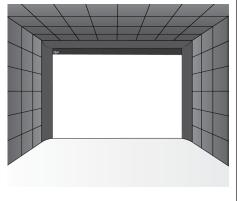
When planning a golf simulator for a new build, consider using plywood on the walls and ceilings to simplify panel installation. It's a gamechanger, streamlining the trickiest part of the installation—securing cleats into study or relying on wall anchors.
