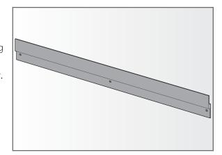
Install Cleat: Use a level and pencil to mark the cleat holes.
