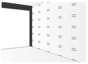
Stud Location: If you don't have plywood walls and ceilings, use a stud finder and laser level to identify and mark stud locations. This step streamlines cleat installation.
