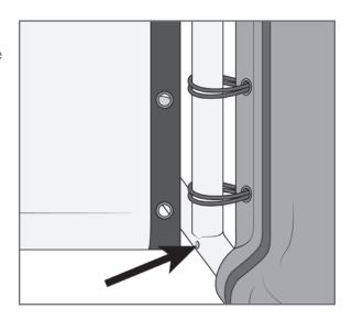
On one side, insert the cable through the fitting. Secure the cable with 4 turns of the cable receiver. Repeat on the other side.
