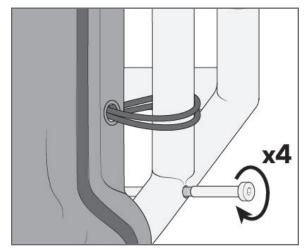
Continue tightening each end of the cable, until the cable is taut. Use a pliers to hold the cable and prevent it from spinning, while using 3/16" Hex key to tighten the receiver.
