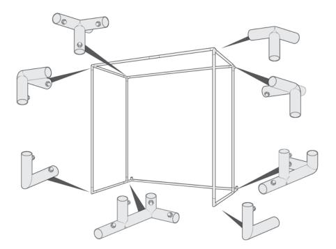
Using the Frame Assembly Sheet included with this enclosure, construct your frame.
