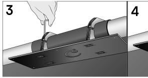
Fully tighten both sides of the clamps evenly to secure the clamps in place.
