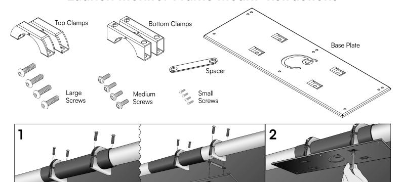
To start, pull back the fabric flap on your Pro enclosure's ceiling pipe where you plan to mount the launch monitor. Put the clamps over the pipe fitting and loosely secure the large screws. If one clamp is off the fitting, use the spacer between the clamp and base plate to level the mount.
