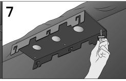
Secure the launch monitor mount to the base plate with the small screws.
