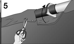
Wrap the flap around the pipe. Then cut slits where the clamp's screw holes are located. Do not cut the finished edge of the flap.
