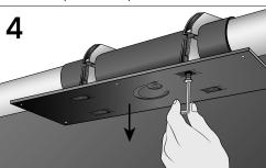
With the clamps in place, remove the base plate by unscrewing the medium screws.
