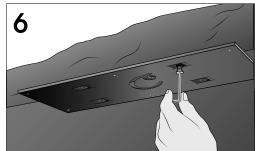
Reattach the base plate to the clamps and tighten with the medium screws.
